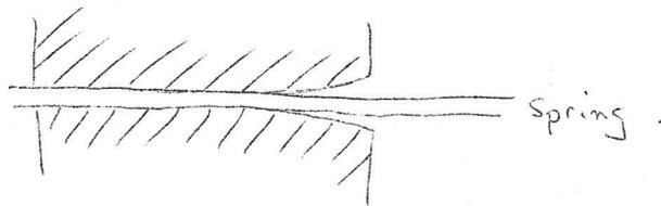
avoiding the stress concentration and secondly, we can use one of the new non-ferrous alloys which are far less susceptible to work hardening under these sort of conditions.
