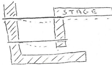
(he scrawls in biro on the representative's last 6F catalogue) surely cannot be satisfactory for a microscope F.A. movement because it is not rectilinear? The horizontal movement must be troublesome when focusing.
